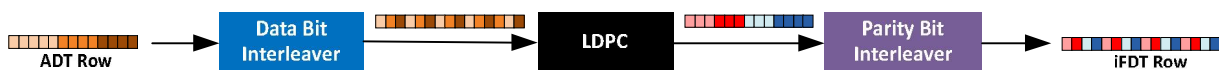
Figure 46: Outer FEC process with bit interleaving of the ADT row before LDPC encoding and bit interleaving of the generated parity bits before writing them into one row of the iFDT. The bit interleaver is simply a block interleaver with the number of columns equal to the data spreading factor B and parity spreading factor S , for data and parity interleaving, respectively.
