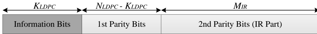
Figure 36: Extended 8k LDPC codeword with incremental redundancy. K_{LDPC} 2160 bits, N_{LDPC} 4320 bits, M_{IR} 4320 bits.
