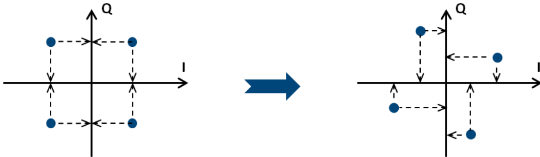
Figure 9. QPSK non-rotated constellation (left) and QPSK rotated constellation (right).
