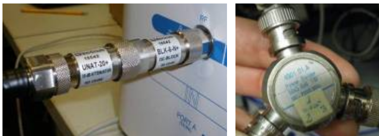
Figure 2.8.5. Laboratory accessories for T2-Lite FEFs laboratory test (attenuators, DC blockers and splitters)
