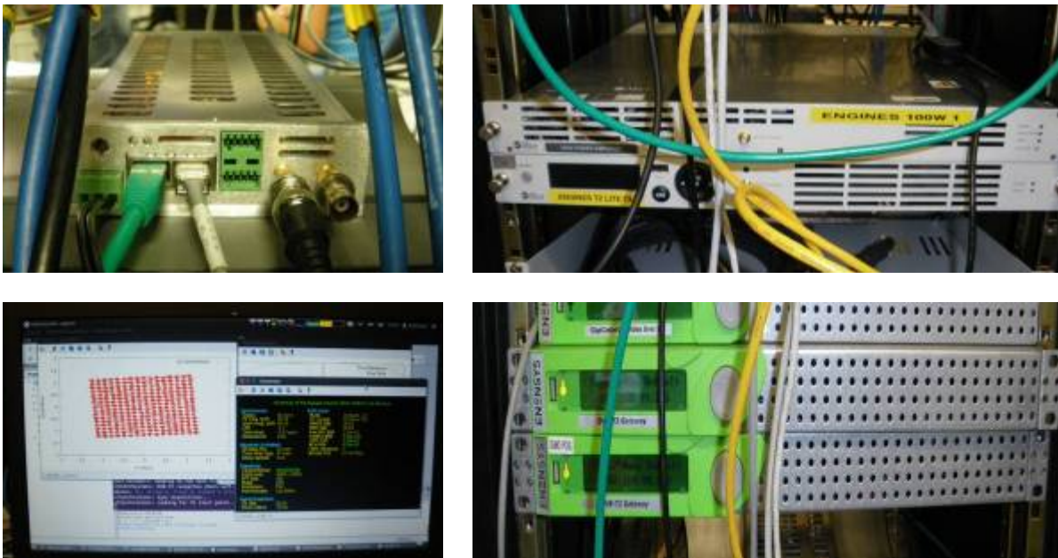
Figure 2.8.1. Prototypes under test in T2-Lite FEF evaluation (TeamCast modulator, Mier transmitter, UPV/EHU demodulator and ENENSYS gateway)
