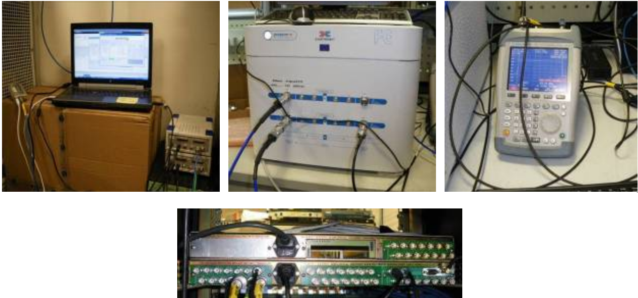
Figure 2.8.4. Additional equipment for T2-Lite FEFs laboratory test (TS players, TUAS channel simulator, spectrum analyser and GPS PPS generator)
