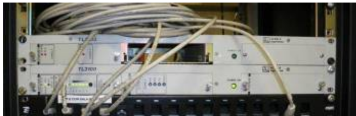
Figure 2.9.4. Additional equipment for Mixed T2 and T2-Lite laboratory test (channel simulator control screen and GPS PPS generator)
