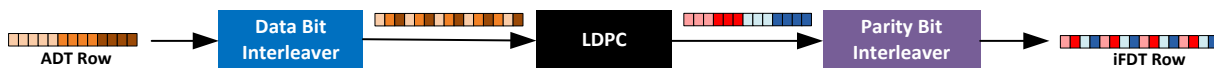
Figure 31: Outer FEC process with bit interleaving of the ADT row before LDPC encoding and bit interleaving of the generated parity bits before writing them into one row of the iFDT. The bit interleaver is simply a block interleaver with the number of columns equal to the data spreading factor B and parity spreading factor S , for data and parity interleaving, respectively.
