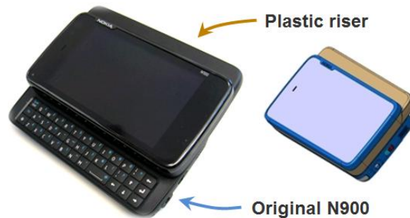
Figure 111. Spectrum sensor prototype implementation on N900 mobile phone.
