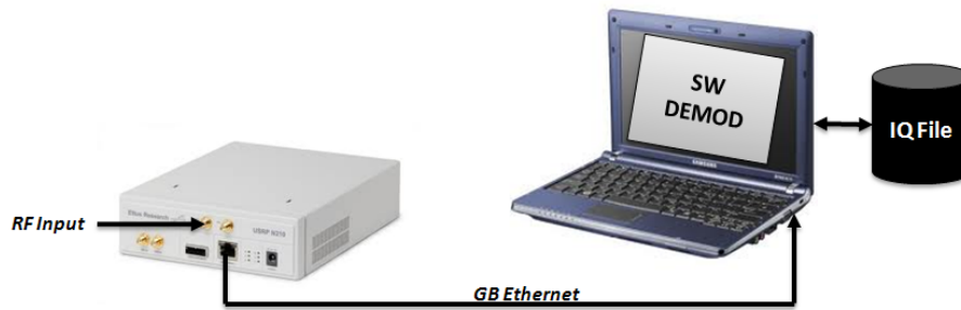
Figure 2. Operation with the USRP module
