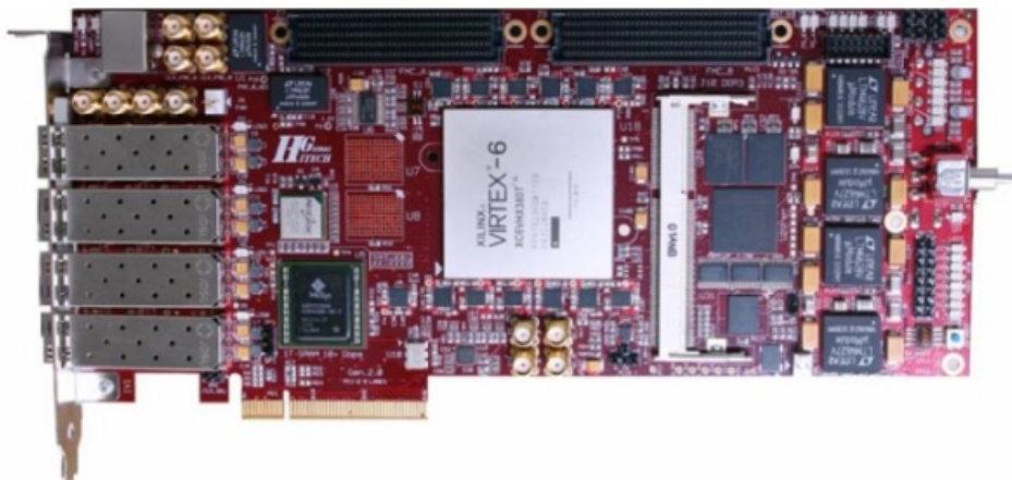
Figure 2: HTG-V6HXT-x8PCIE FPGA board.
