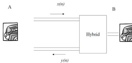
However, due to imperfect balancing of the hybrid (today mobile device), there is always a echo from the insignal  $x(n)$  to the outsignal  $y(n)$  back the talker. If the delay of this echo is more than 100 ms, it starts to disturb the communication. The delay is nowadays often increased due to digital techniques, due to increased buffering of data in the overall system. Hence, to minimize the echo in the outsignal  $y(n)$  is important.
