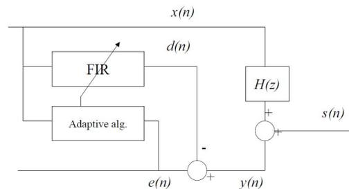
The crucial element in adaptive filters are the adaptive algorithm. Least Mean Square (LMS) algorithms are often used in this context. In this exercise we will use Stochastic Iteration Algorithm given by
