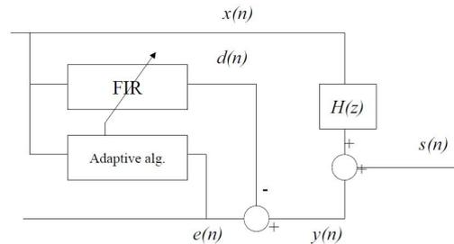
The crucial element in adaptive filters are the adaptive algorithm. Least Mean Square (LMS) algorithms are often used in this context. In this exercise we will use the Stochastic Iteration Algorithm given by
