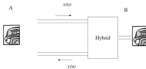
However, due to imperfect balancing of the hybrid, there is always an echo from the incoming signal  $x(n)$  to the outgoing signal  $y(n)$  back to the talker. If the delay of this echo is more than 100 ms, it starts to disturb the communication. The delay is nowadays often increased due to digital techniques, due to increased buffering of data in the overall system.
