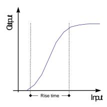
Having determined the rise time (measured in seconds), we can making some simplifying assumptions - calculate the required sample frequency as follows:
