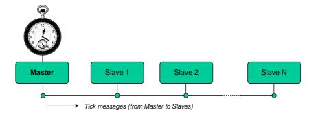
Here we have one, accurate, clock on the Master node in the network.
