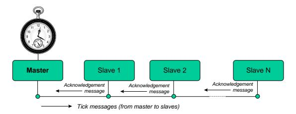
1. Timer overflow in the Master causes the scheduler 'Update' function to be invoked. This, in turn, causes a byte of data is sent (via the CAN bus) to all Slaves:
