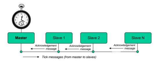
This is a 'time division multiple access' (TDMA) protocol, in which the acknowledgement messages are interleaved with the Tick messages.
