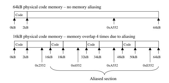
If you want to increase the chances of detecting program-flow errors using this approach, you need to use the maximum amount of (code) memory that is supported by your processor. In the case of the 8051 family, this generally means selecting a device with 64 kB of memory. Clearly, this choice will have cost implications.
