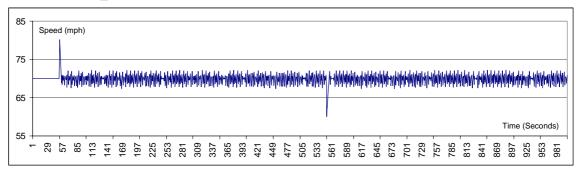
The results of this experiment suggest that a value of KP = 0.5 will be appropriate (that is, half the value used to generate the constant oscillations).
